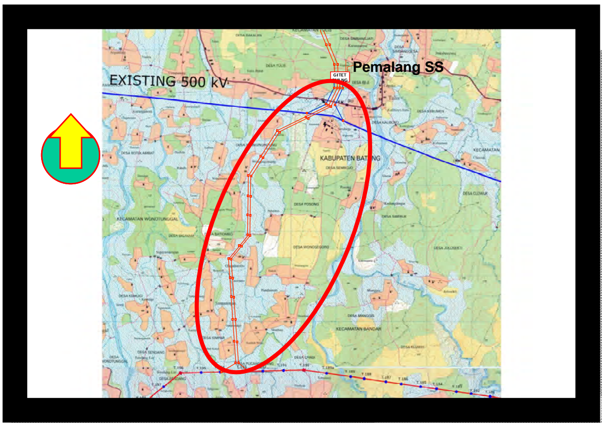
Figure 9. 3 Parallel Route of Double Circuit Towers to Pemalang S/S
