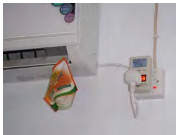
Figure 2.2.1-3 Socket-Type Watt-hour Meter (Measuring Electricity Consumption by Appliance)
