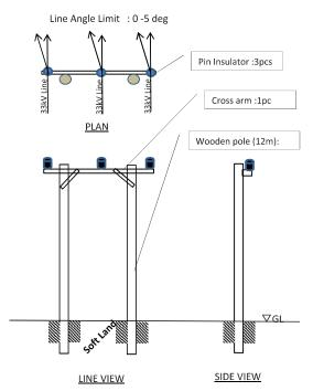
$\mbox{Pole Type W} \\ \mbox{DWG No. T-16} \qquad \mbox{Intermediate Pole (area to be flooded)}$
