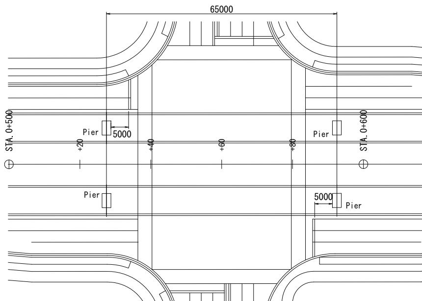
**Figure 2.2.14 Pier locations of Main Bridge at TAZARA Intersection**
