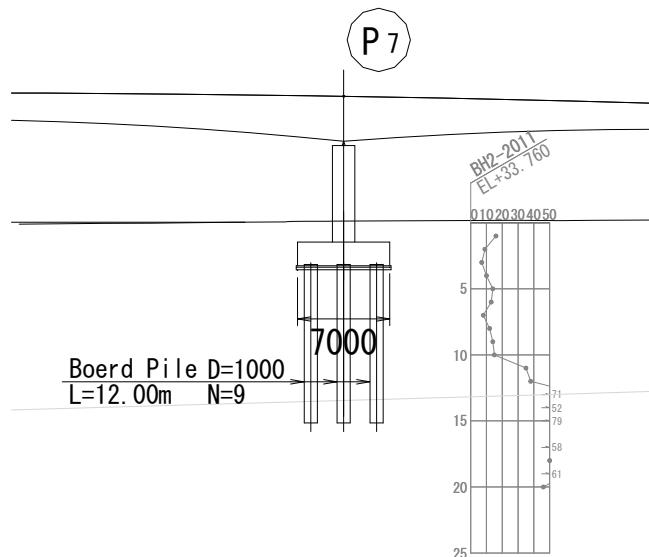
**Figure 2.2.17 Cast-in-place Concrete Pile (P7)**
