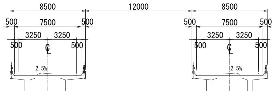
**Figure 2.2.12 Typical Cross-section for F/O Bridge**
