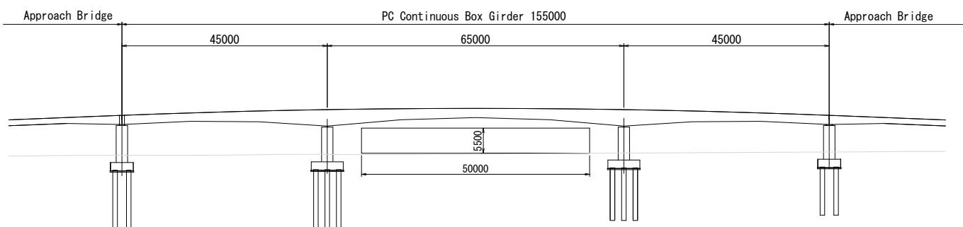
**Figure 2.2.15 Profile of Main Bridge**
