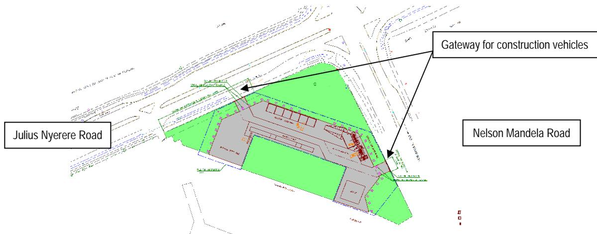
**Figure 2.2.18 Construction Yard**
