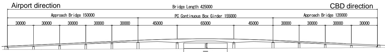
Figure 2.2.16 Profile of Approach Bridge
