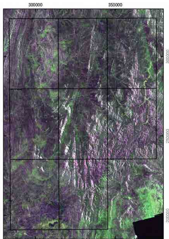
Figure 7.11 Polarimetry composite image of PALSAR L4.1 data (RGB=HH,HV,VV)
