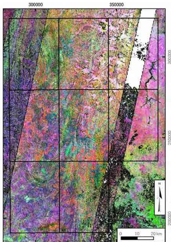
Figure 5.4 Band ratio image of ASTER L3 data (RGB=B4,B6,B1)
