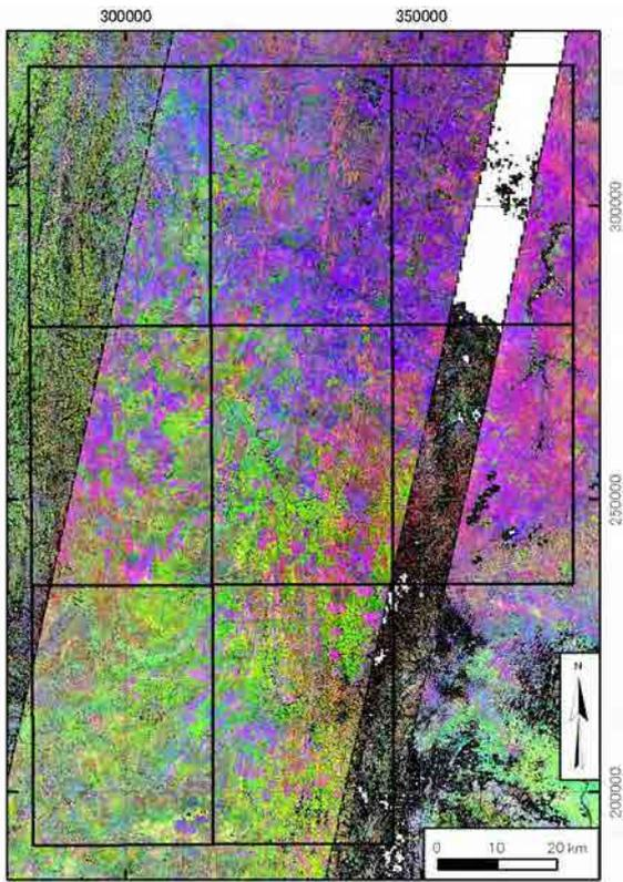
Figure 5.5 Band ratio image of ASTER L3A data (RGB=B5/B6, B6/B8, B5/B4)
