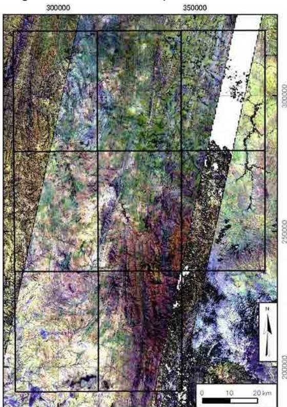
Figure 5.3 Band composite image of ASTER L3 data (RGB=B3,B2,B1)
