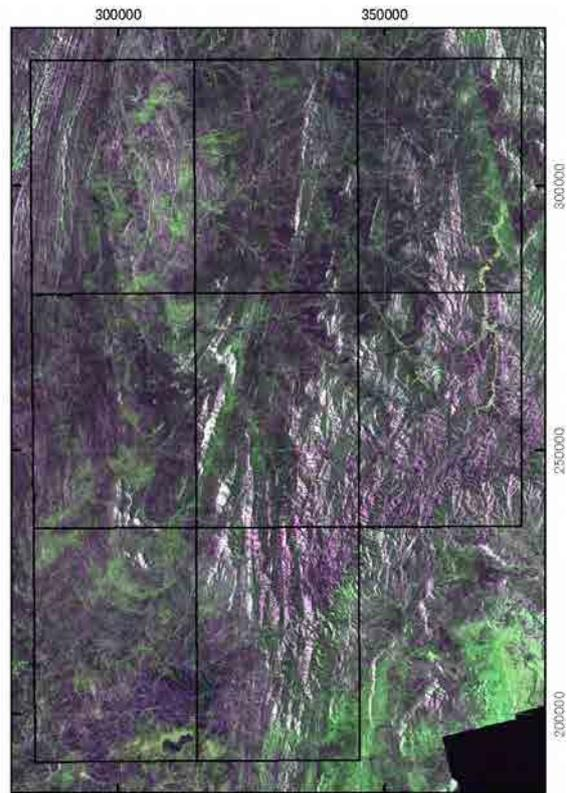
Figure 5.10 Polarimetry composite image of PALSAR L4.1 data (RGB=HH,HV,VV)
