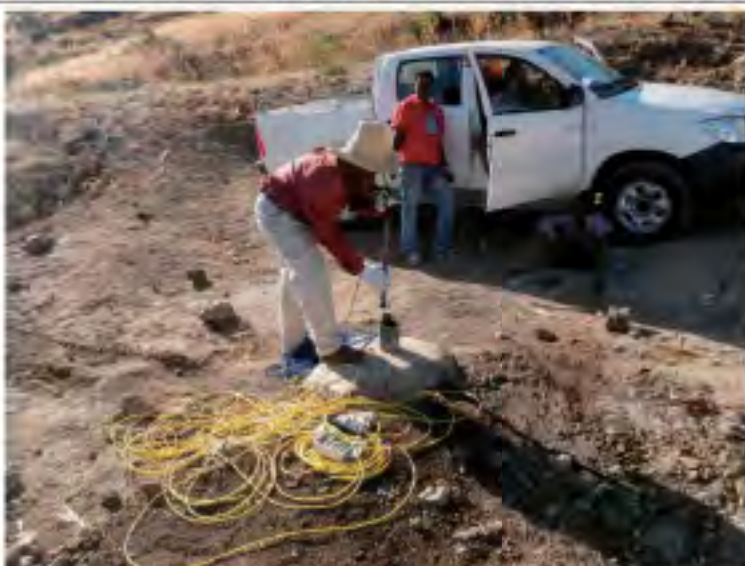
2011.12.28 B28_10 Groundwater resistivity logging
