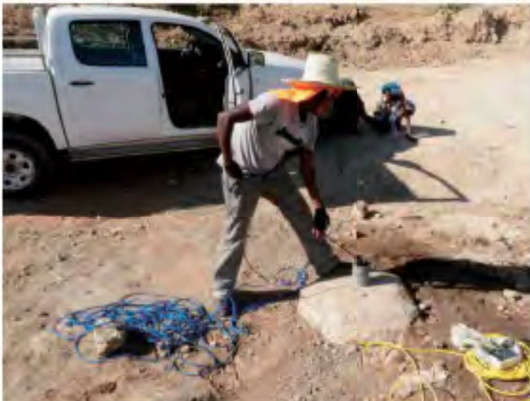
2011.12.28 B28_10 Groundwater resistivity logging
