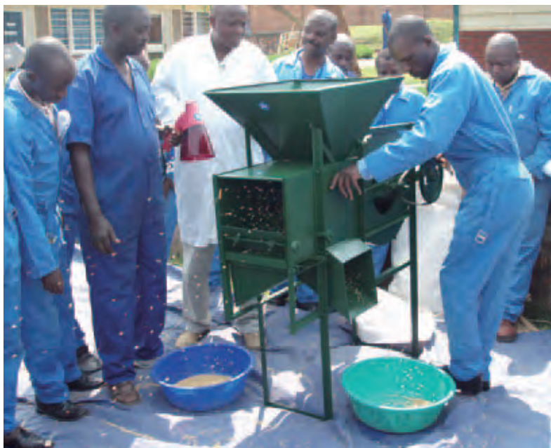
Engineers testing the fanning mill (Rwanda)
