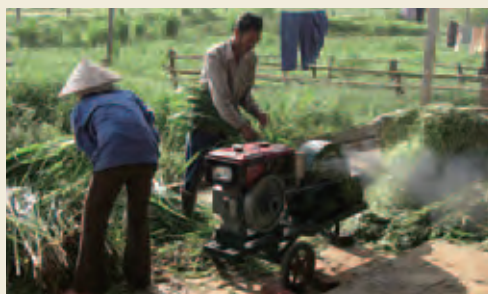
The use of grass chopping machines that make tough grass easier for cows to eat spread rapidly after they became less expensive by having them manufactured by local blacksmiths.
