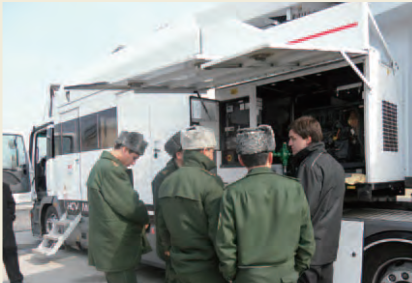
Vehicle-mounted large-scale scanner provided for use with cargo (Oybek Customs Check Point).
