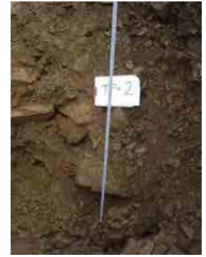
Dmax ≈ 300mm, air void is large and loose Photo 3: Test Pit 1
