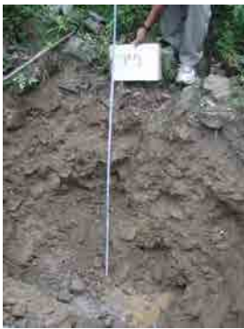
Cobble of Dmax 200mm is distributed on surface as depth 0.1m. Gravels of Dmax 150mm in depth 0.1 or more.
