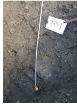
Dmax ≈ 200mm, air void is smaller than other pits
