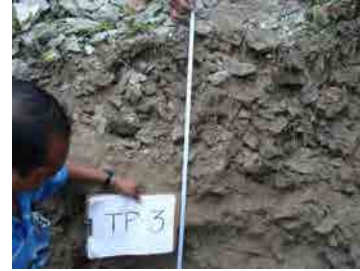
Gravels of Dmax ≈ 30~50mm are distributed on ground surface of depth 0.6m or less. Gravels get fewer in lower layer. All layer is loose.
