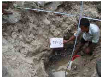
Cobble of Dmax 300 is distributed in depth 0.0~0.3m. Depth 0.3~1.3m is gravels of Dmax 150mm. Depth 1.3 or more is sand and gravel, and springwater
