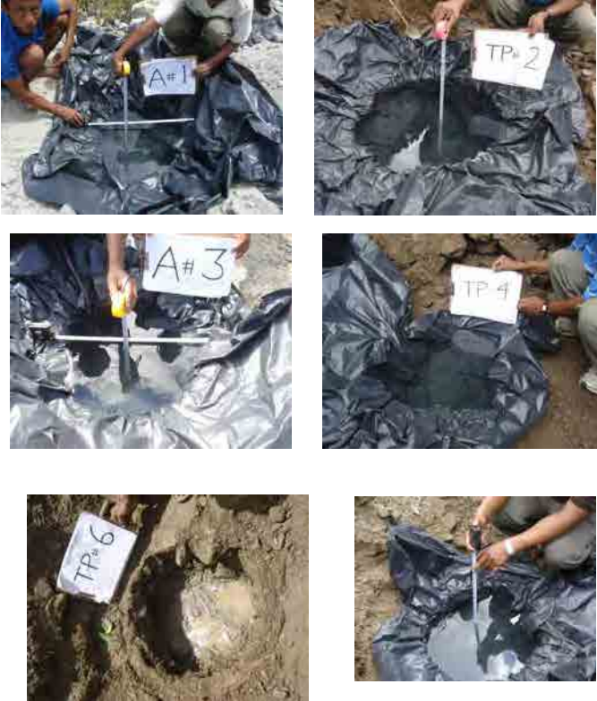
Photo 11: IN-SITU DENSITY TESTS BY WATER REPLACEMENT METHOD
