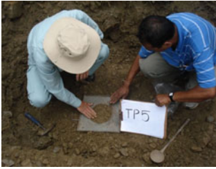
Photo 10: In-situ Density by Sand Cone Method
