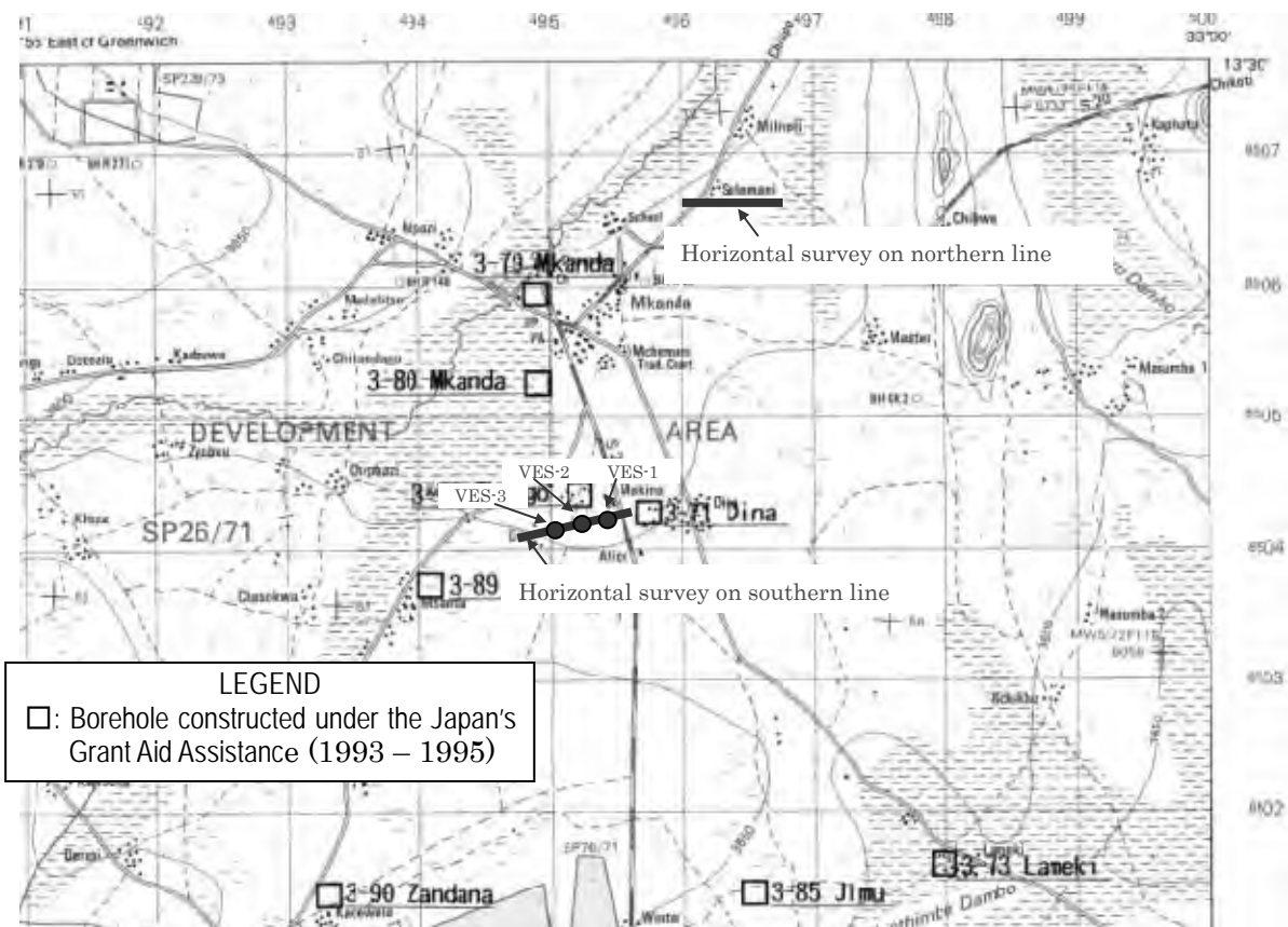
Figure A6-1-20 Location Map of Horizontal Geo-electric Survey
