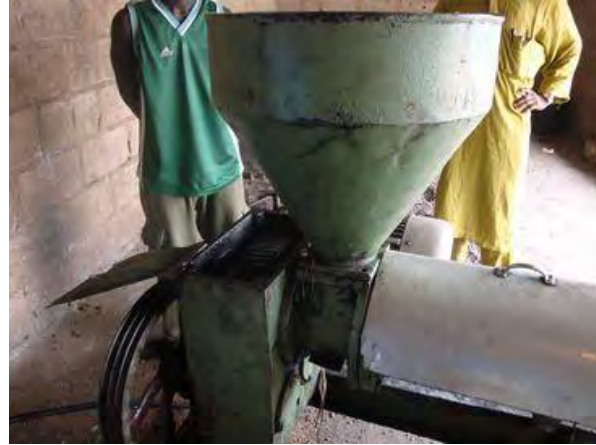
Gear box and feeder shaft
