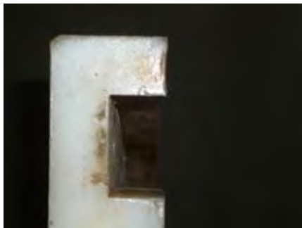
Photo 3.2-6 Teflon segments (replaced)
