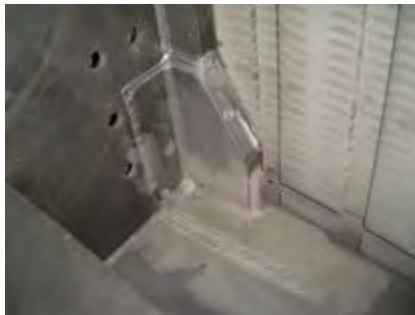
Photo 3.1-4 Repaired rotor Spider (2G5)
