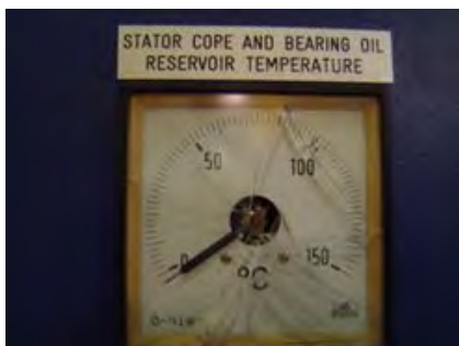
Photo 3.1-14 Indication error of resistance thermal detector (RTD) thermometer
