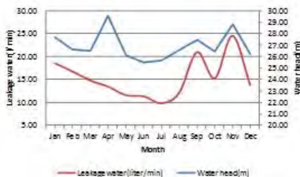
Figure 3-9 Leakage Water Powerhouse and Intake
