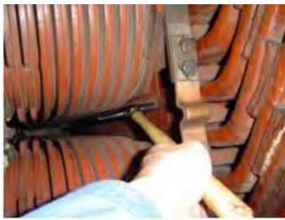
Photo 3.1-3 Tapping of stator wedge
