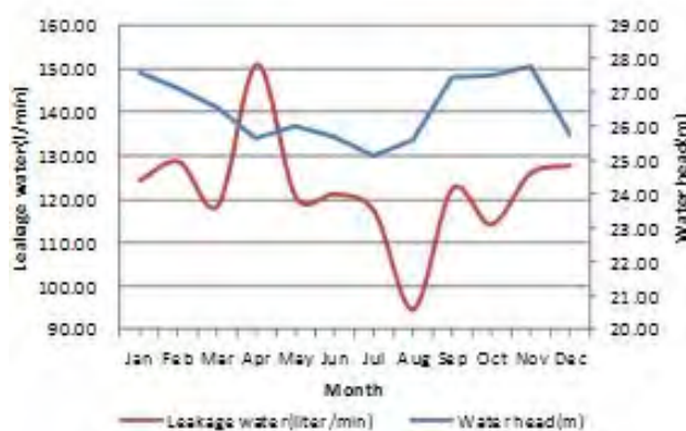
Figure 3-8 Leakage Water Auxiliary Dam 3
