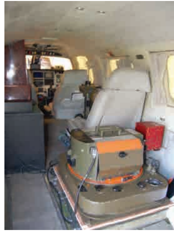
Picture 3-7 Aerial camera Installed on airplane
