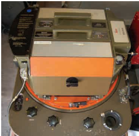
Picture 3-6 Aerial Camera Leica RC30
