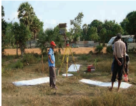
Photo Control Point Survey (GPS Survey)
