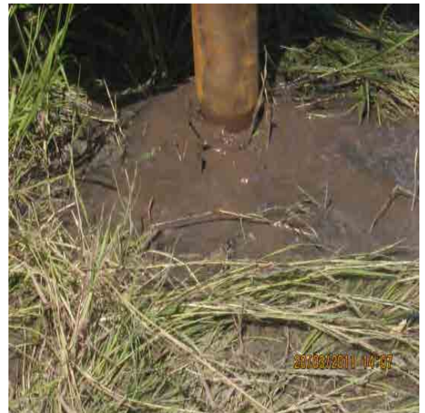
Wash Boring at 8.0 meters
