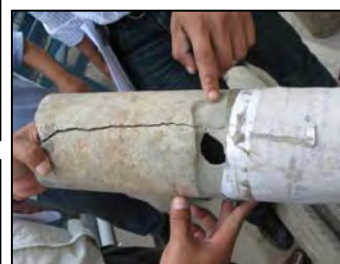
Photograph-3: Reduction with lead from asbestos cement to PVC in Comas. No suitable accessory.
