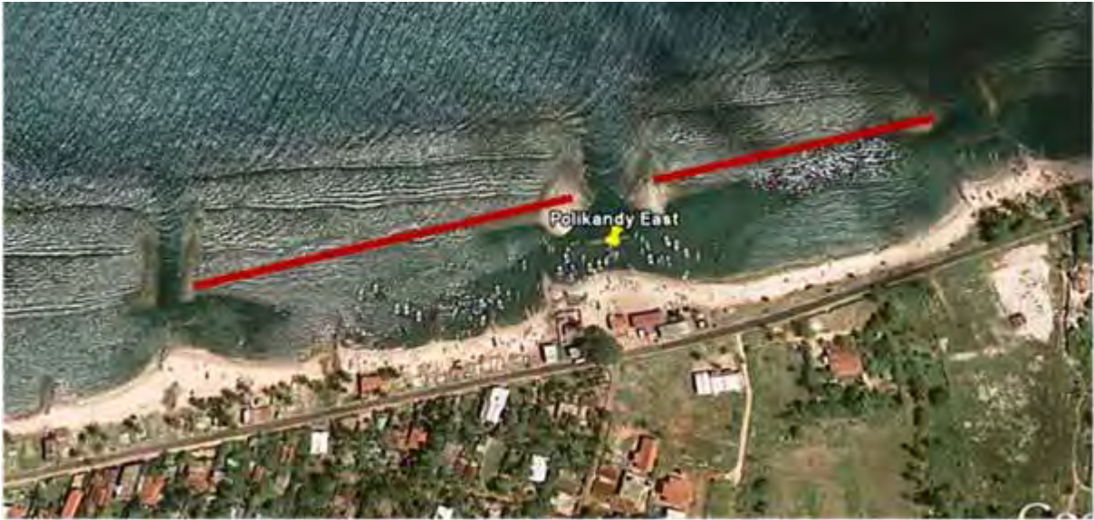
Figure 6.12: Polikandy East: Anchorage Layout
