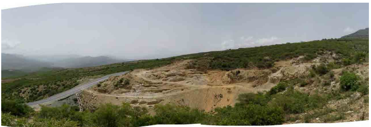
Photo 3. 9.33 Quarry located on the right channel bank (sediment runs off into the channel from the quarry)
