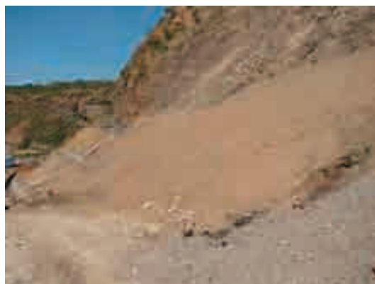
Photo 4.4.6 Fine tuff to lapili tuff with partly sandy tuff in the Pyroclastic rock (2)
