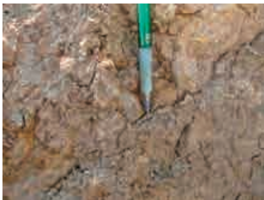
Photo 4.4.15 Tuff, which might be highly weathered basalt, under the Basalt
