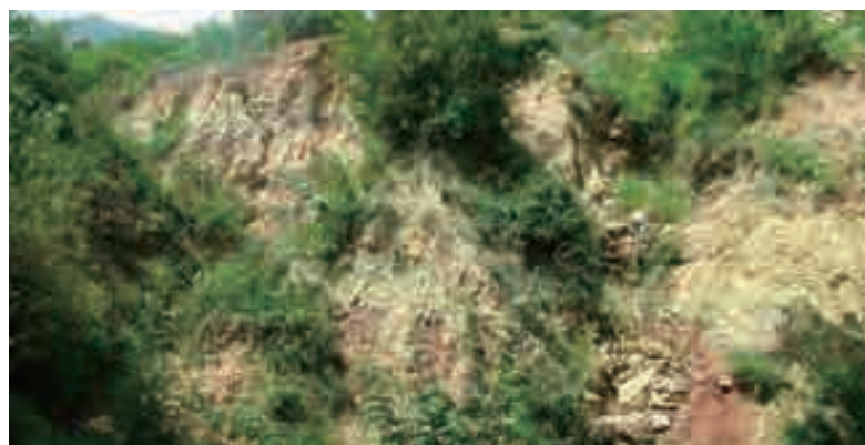
Photo 4.4.21 Reddish and greenish silt and shale layer on the lower slope of Filiklik(STA.11+400)
