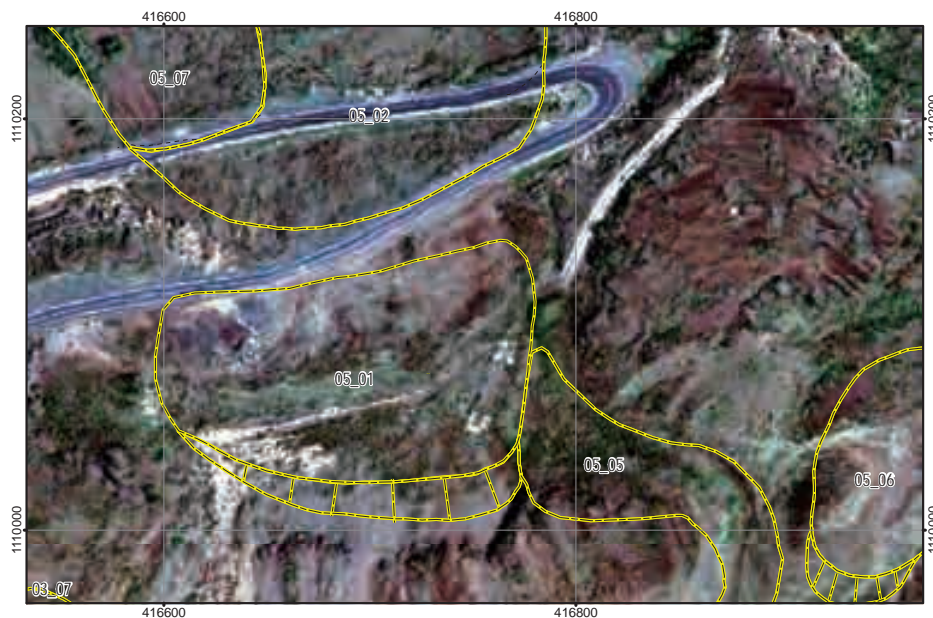
Figure 4.3.1 Examples of old landslides (L/S05-01)
