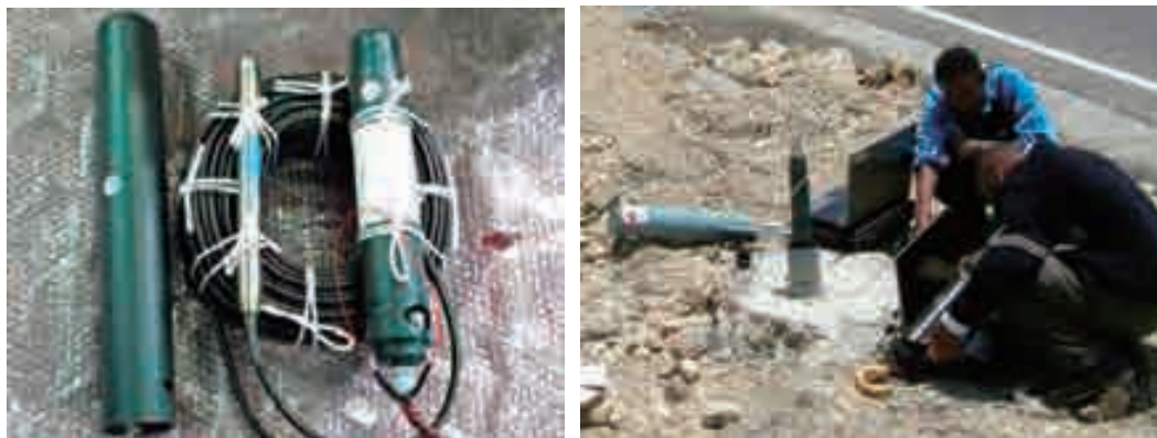
Photo 3.5.5 Device of Groundwater Level Measurement
