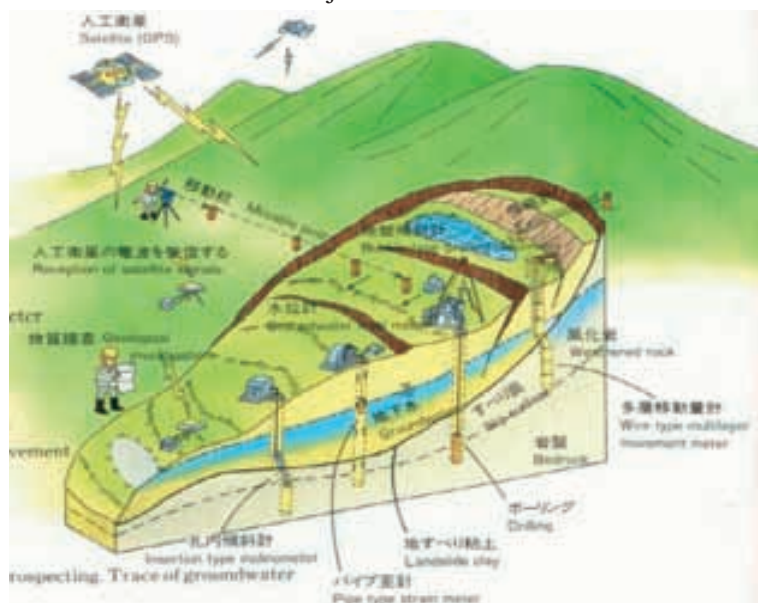
Figure 3.5.1 Various kinds of devices for landslide monitoring
