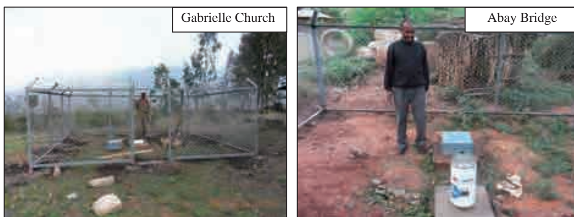
Photo 3.1.2 Newly Installed Rain Gauge Station
