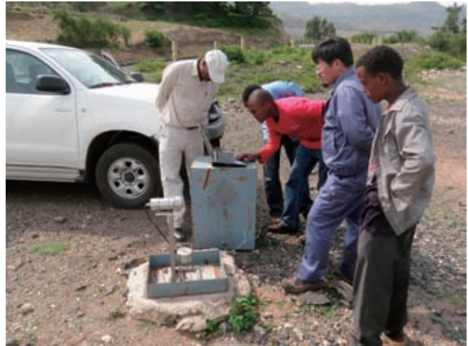
Monitoring data collection of borehole extensometer, 21 st Jun. 2011
