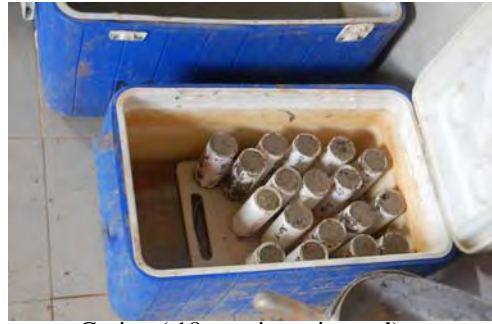
Curing ( 18-specimen in total)
