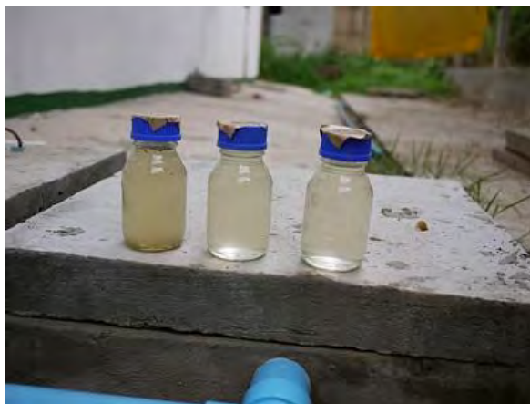
SBS: From the left, inflow tank, intermediate tank and outflow tank
