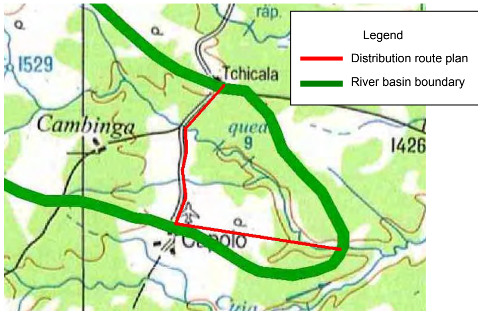
Fig. 3.2-11 Distribution Line Route Plan from Luvolo River Site to Chicala Village
