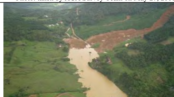
Earth flow occurred in November 2008 in northern Benedito Novo. Earth flow included mainly yellow-reddish soil with some gneiss debris. Cunha river was temporarily dammed and a natural slide dam was formed. At the downstream of the natural dam is the municipality of Rio dos Cedros.
