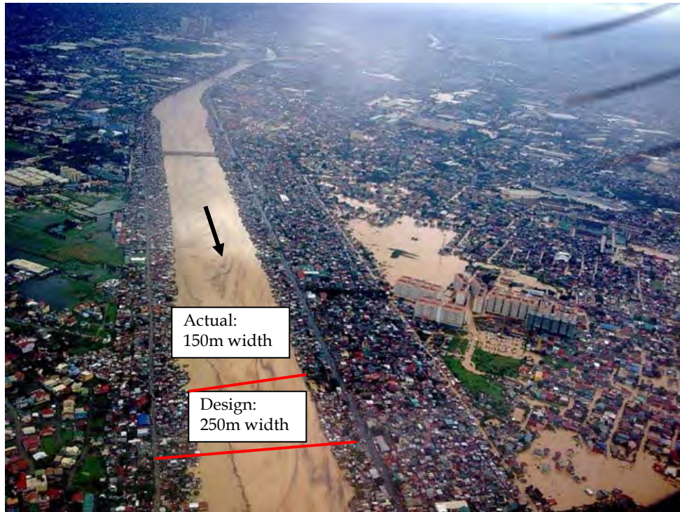
(Manggahan Floodway; 2 days after “Ondoy”. There are existing structures of informal settlers inside of channel between the both roads on the banks.)
