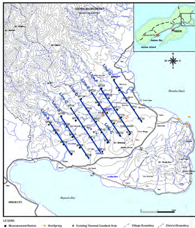
Fig.III-2-40 Location of Resistivity Section Lines
