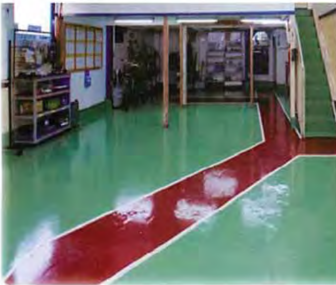
Fig.3 The walking way and the working area are separated to avoid traffic and for employee safety
