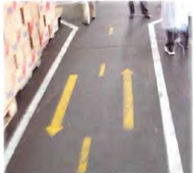
Fig.3 The walking way and the working area are separated to avoid traffic and for employee safety
