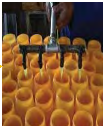
Elimination of Muda of motion and transportation by introducing filling hose saves labor force & increase productivity.
