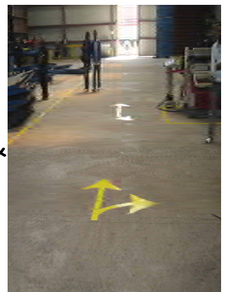
Places for everything from walkways to work areas are well identified, labeled and marked in a standard way through implementation of 5S
