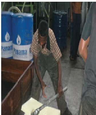
Eliminating Muri (overburden): manual crushing of raw material to semi-automatic crushing machine leading to higher productivity.
