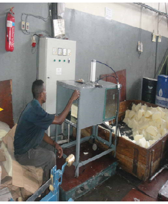
Eliminating Muri (overburden): manual crushing of raw material to semi-automatic crushing machine leading to higher productivity.
