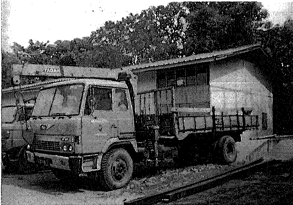
7.5 TON CARGO TRUCK WITH 4 TON CRANE HINO MODEL " FH- 224 SA-NA"
