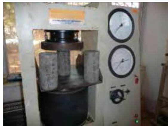
Compressive Strength Test Image
