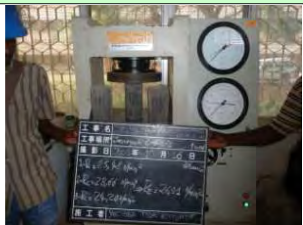
Step6. Concrete Compressive Strength Test
