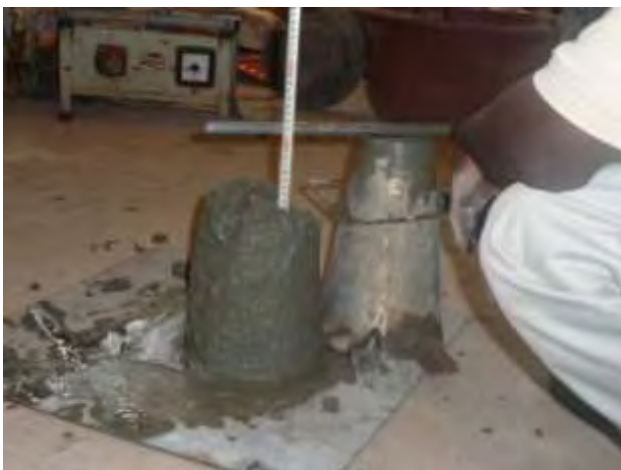
Step3. Check for Moisture Content and Slump
