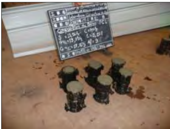
Compressive Strength Test Sampling Image
