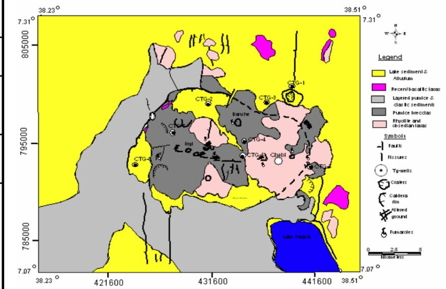
Figure 11, Geological map of Corbetti geothermal prospect (GSE, 1987)
