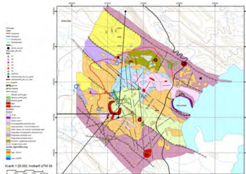
Detailed Geologic Map of the Asal Geothermal Field
