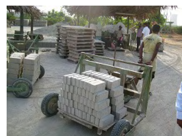
Manufacturing of Sun-Dried Bricks made by Fly Ash
