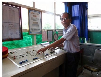
Centralized traffic control (CTC) device as part of auto signaling system (Cipunegara station)
