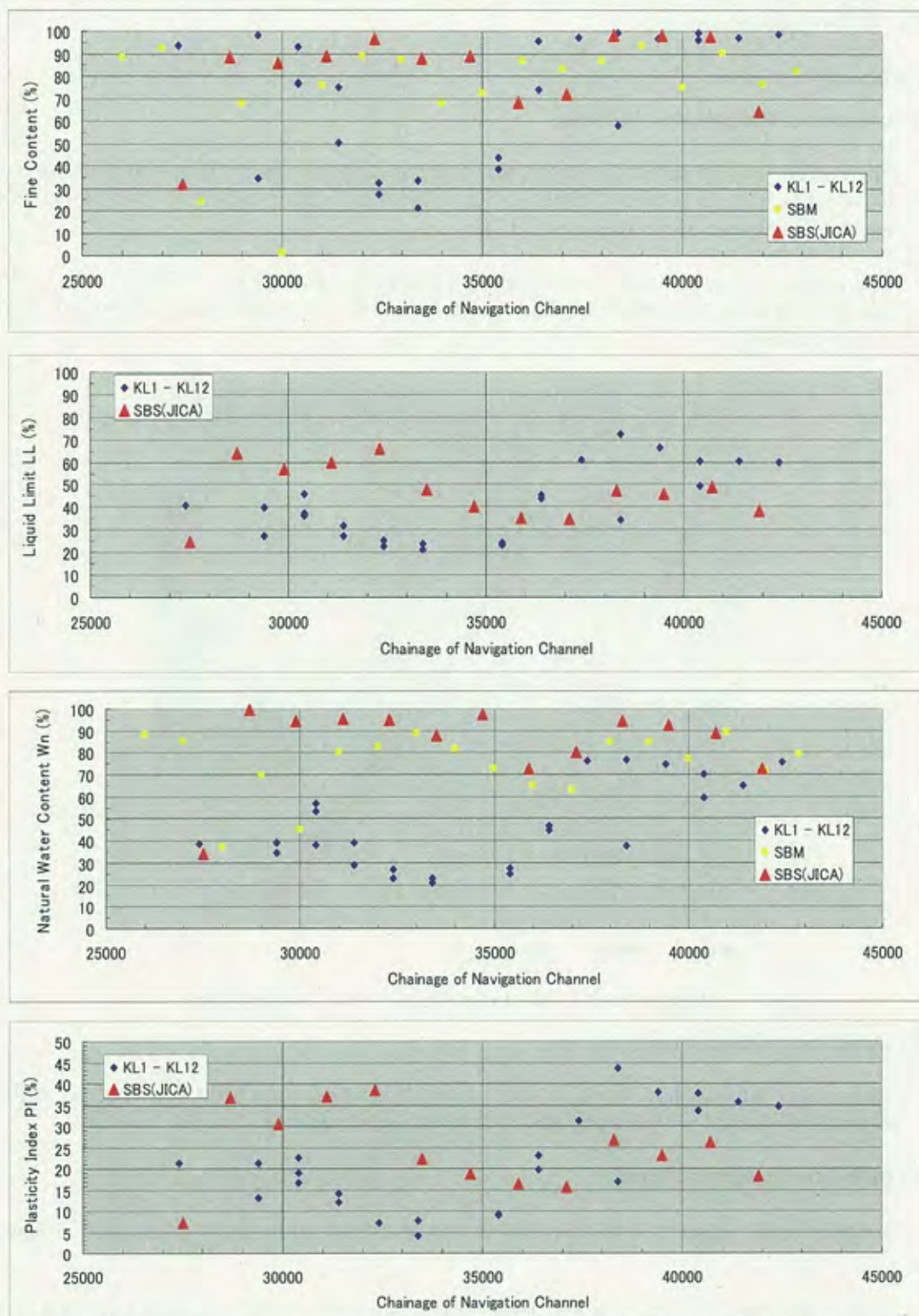
Figure 7.3.26 Physical Property Test Result of Seabed Material along the Navigation Channel
