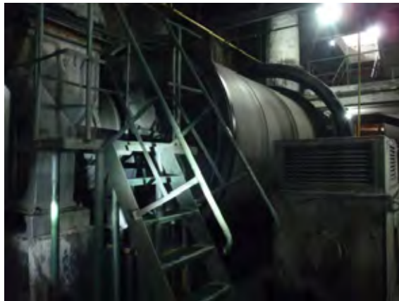
Figure 1.3-13 Affairs of coal pulverization by a mill
