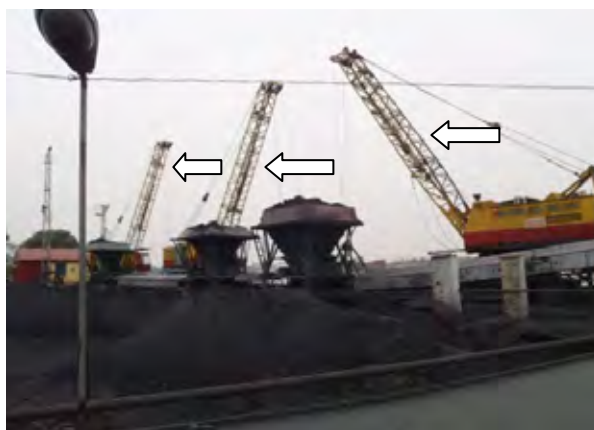
Figure 1.3-3 Features of coal-hoisting installations Arrows indicate crab bucket-type self-propelled cranes.
