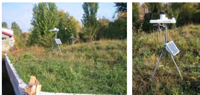
Photo Left : The instrument (left) used for measuring solar radiation and temperature
