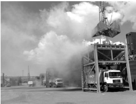
Figure 2.7-14 Dust dispersion from clinker handling
