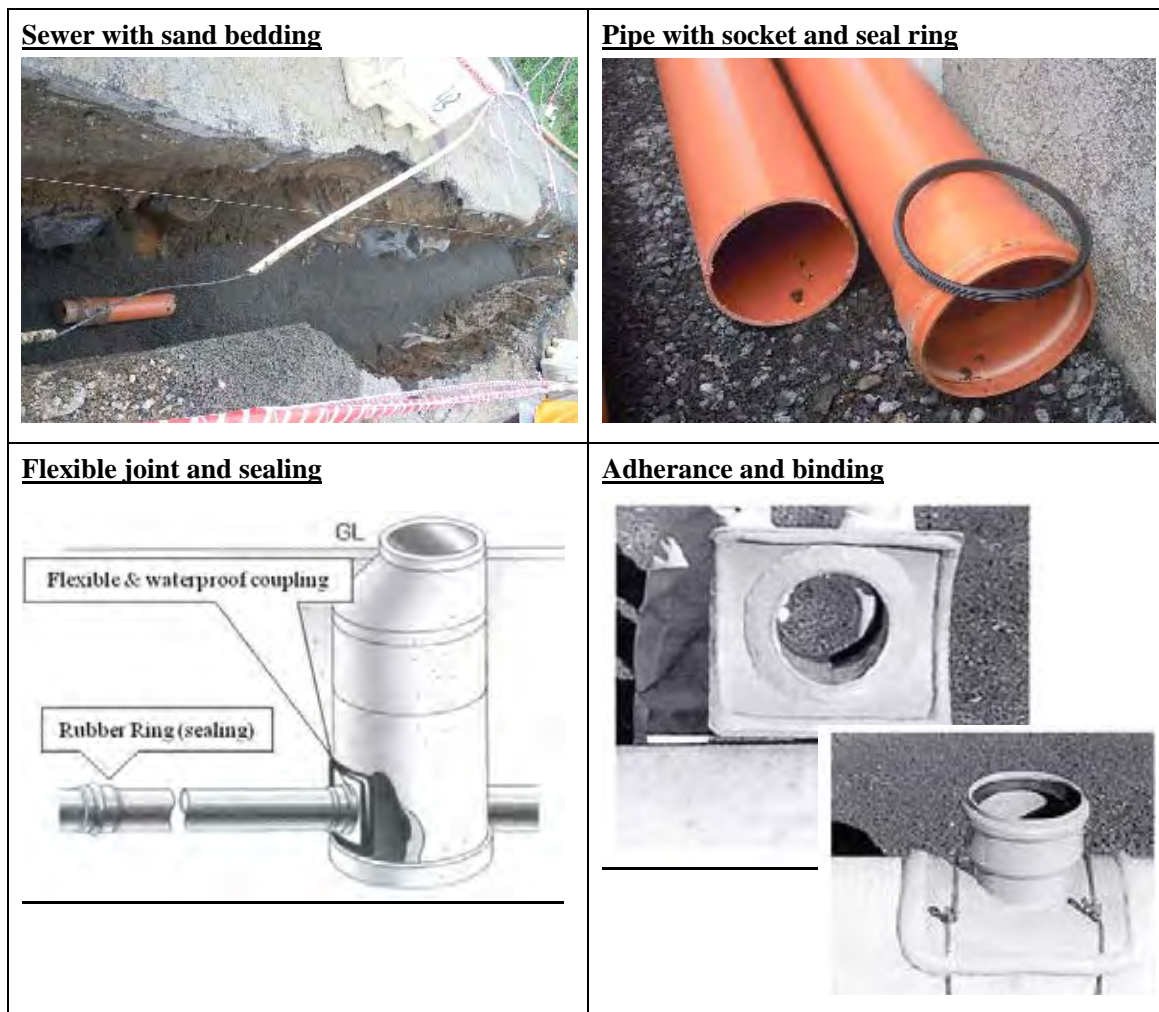
Figure 5.3-4 I/I Mitigation during the Construction Stage (1/2)
