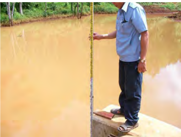
Measuring the thickness of the mud accumulated in front of the intake
