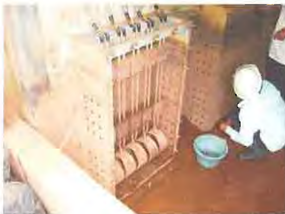
Disassembly inspection of Dummy load
