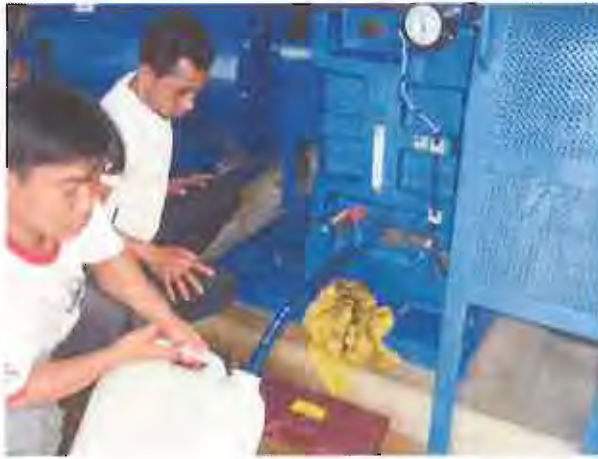
7. Change lub. oil for speed gear
