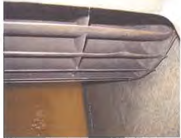
2. Bending portions on runner vanes
