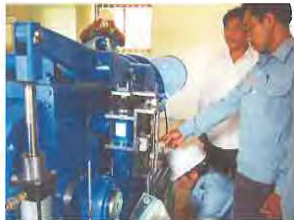
Adjustment of Servo-motor stroke for Guide-vane
