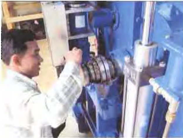
Change of bearing grease
