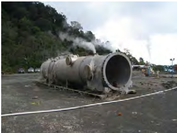
New Separator equipment
