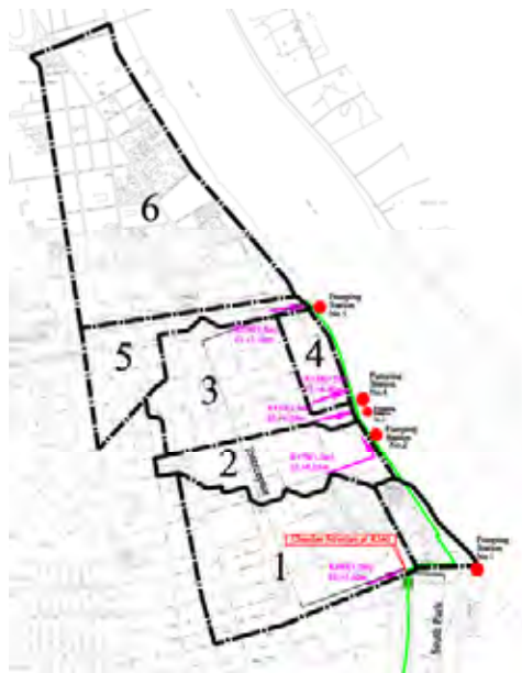
Fig. R 2.2.15 Sub-Basins of Drainage Network in Upstream Area of Chamber at R240
