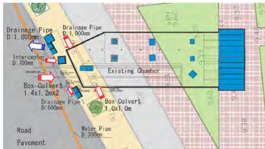
Fig. R 2.2.14 Complicated Drainage Network System near the Old Chamber
