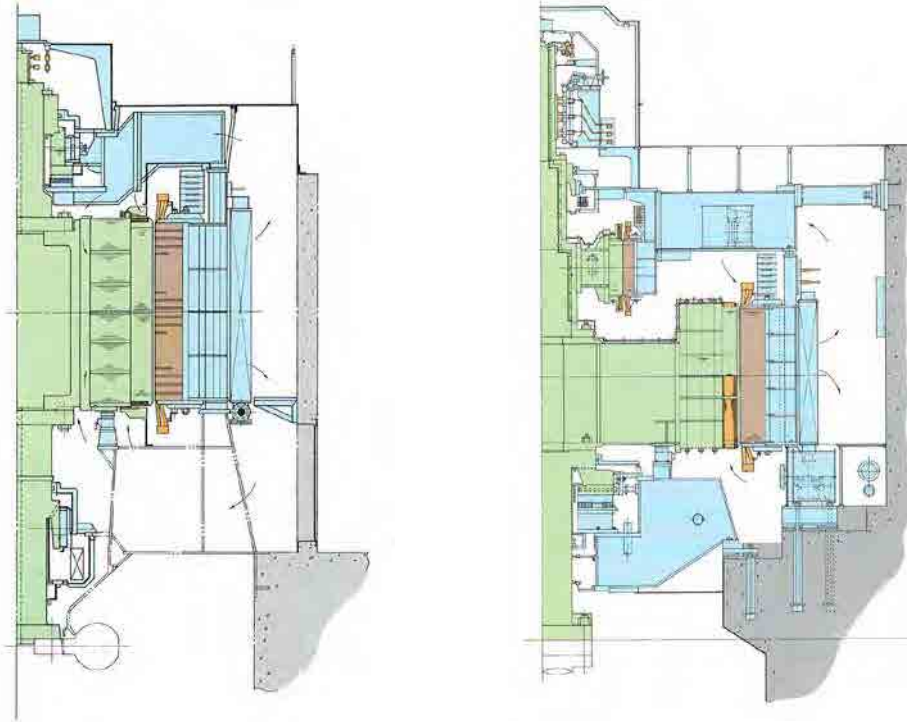
Ventilation by self-ventilation fan
