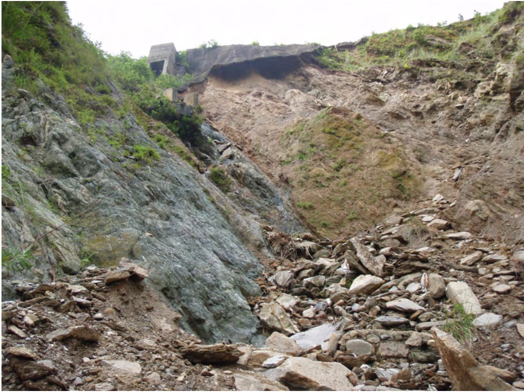
Photo.5-1 A geological boundary between slightly weathered green schist and highly weathered mica schist.
