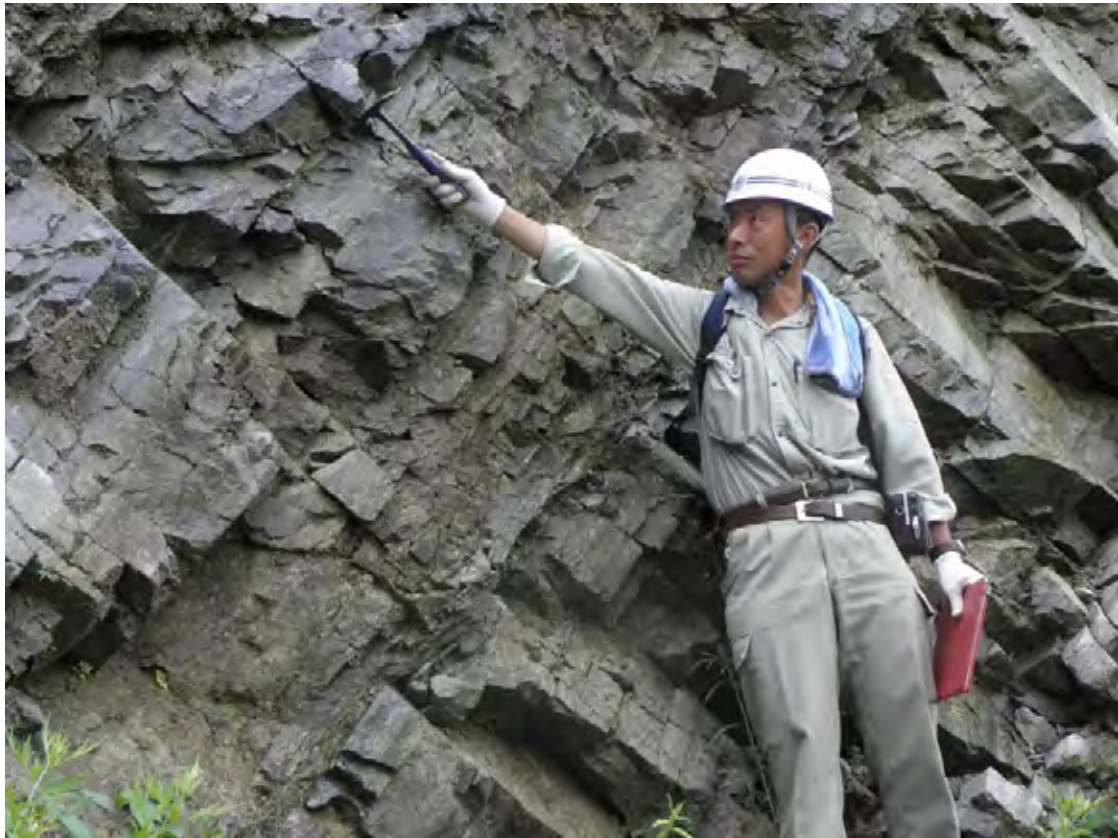
Photo.6 Geological outcrop at Sta.17+600 site. (Cracked Quartz Schist)
